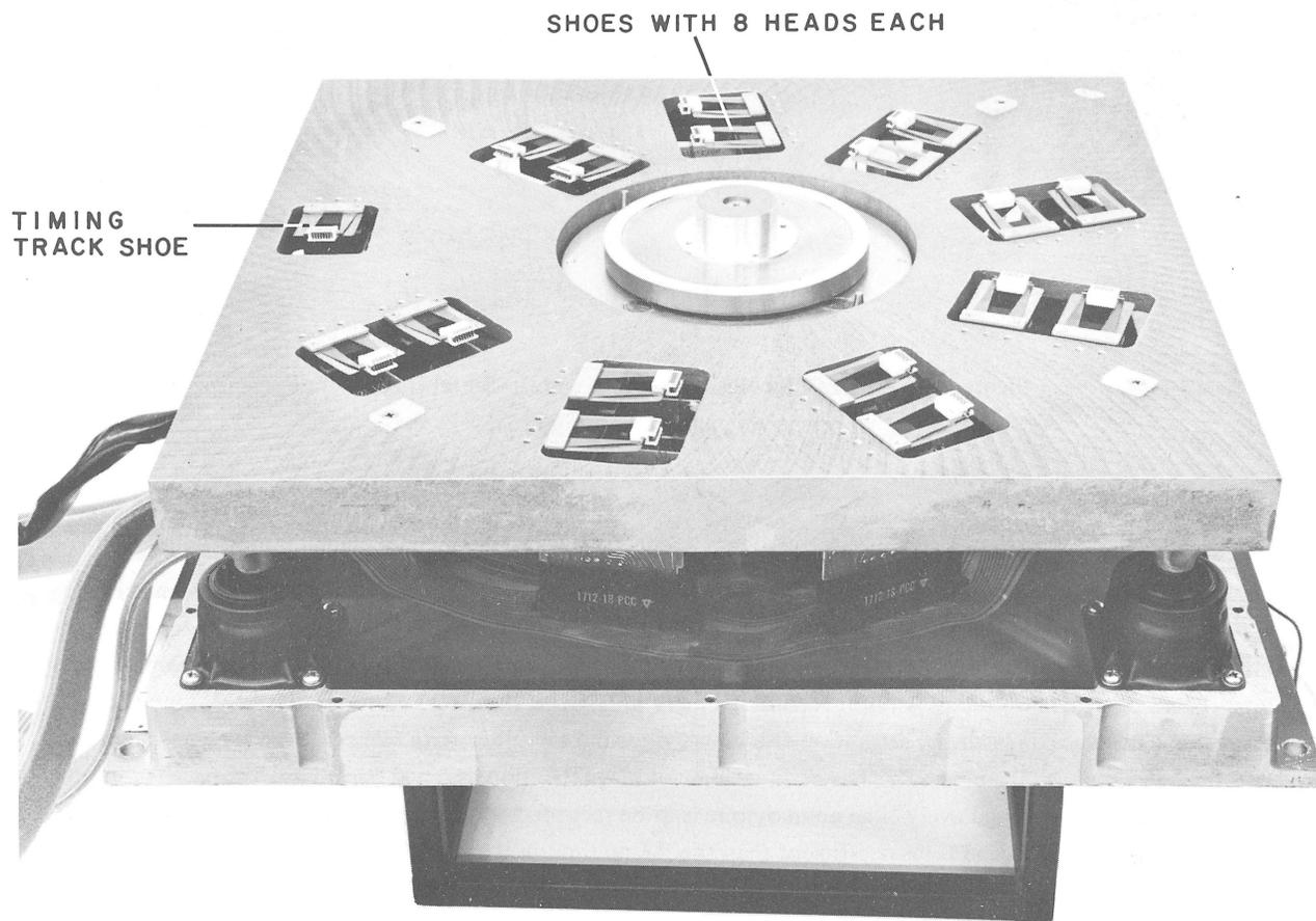
Figure 3-2 Disk Assembly With Cover and Surface Removed
