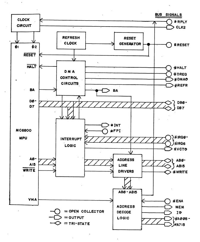
CPU-125 CENTRAL PROCESSING UNIT MODULE BLOCK DIAGRAM
