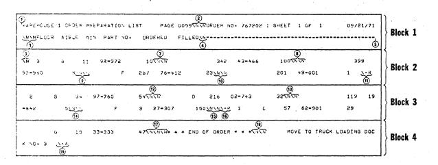
Figure 6-2. Data blocks containing Data and Control Sequences for Printing on a 4310 Terminal.
