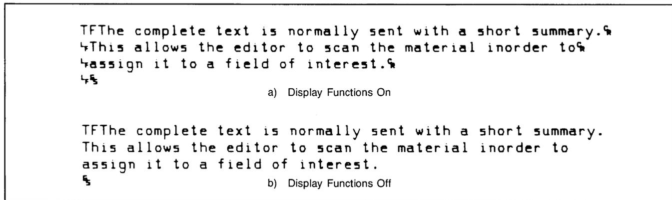
Figure 5-24. Control Character Display On Driver Terminal
