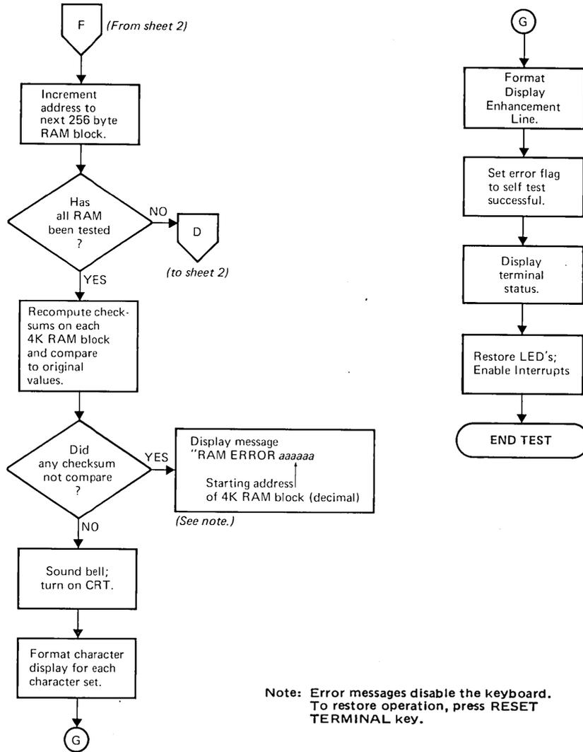
Figure 7-32. Basic Terminal Self-Test Flowchart (Sheet 3 of 3)
