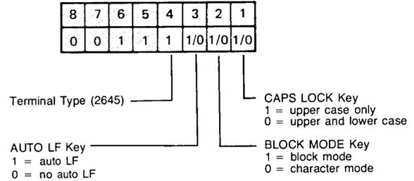
**BYTE 1 KEYBOARD INTERFACE SWITCHES (A-D)**
