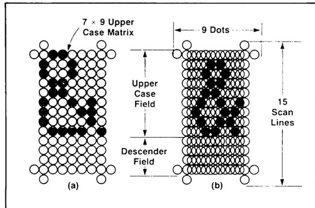
by use of the half-shift. With this type of set the character-to-character spacing of two dots is hardwired. This prevents the design of characters that would form continuous horizontal lines. However, all 15 scan lines of the row are available so that vertically contiguous symbol segments can be designed. An example of this is the three-row-high integral sign found in the math symbol set.
