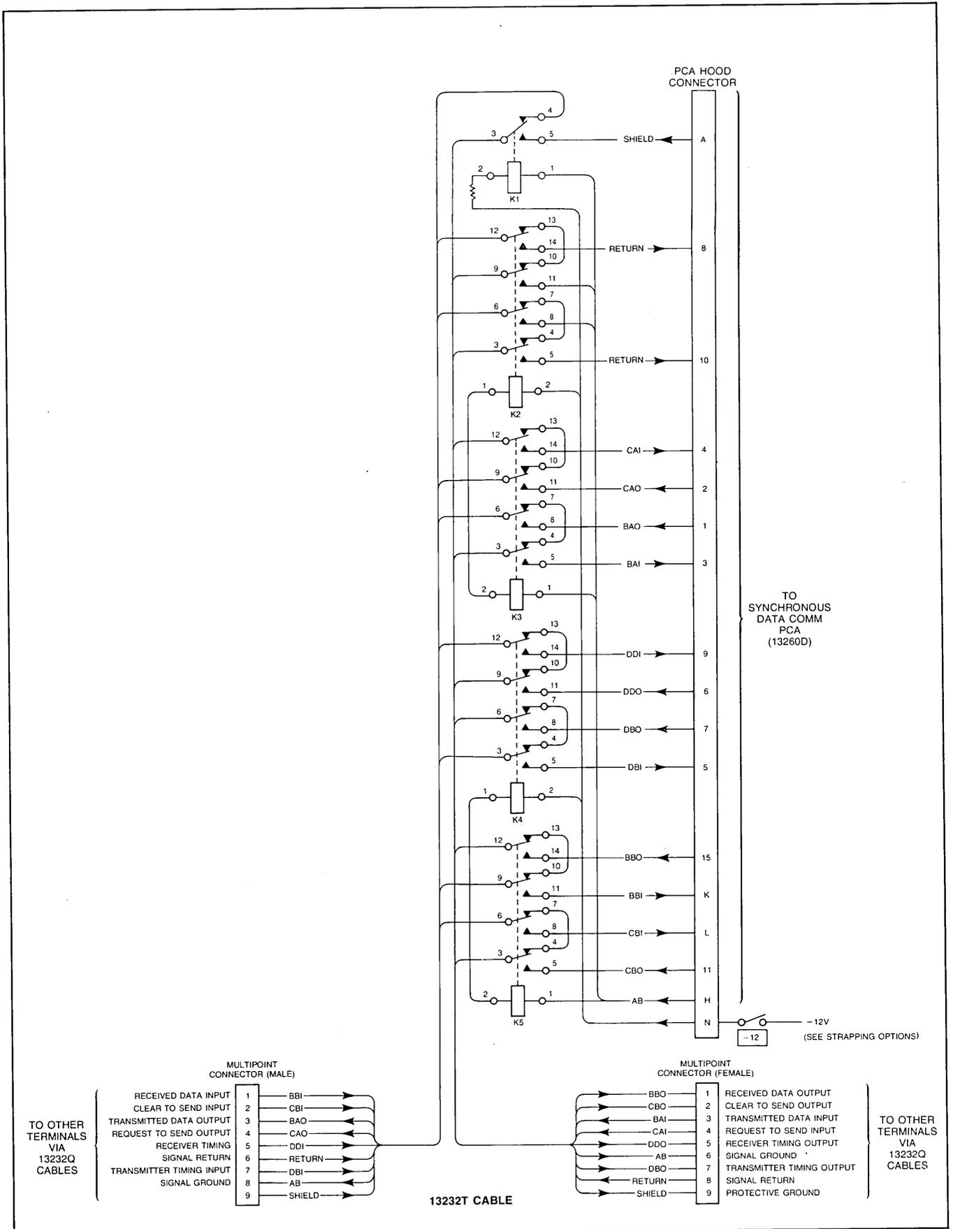
Figure 7-27. Power-Down-Protect Cabling for Synchronous Multipoint Configuration
