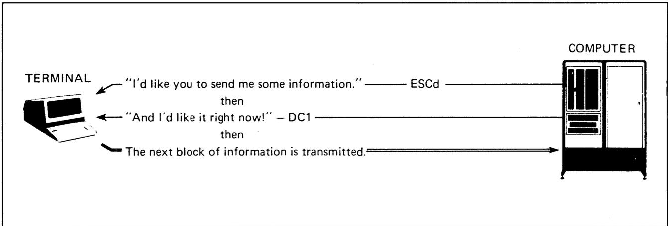
Figure 5-3. Block Transfer Enabled By The Computer
