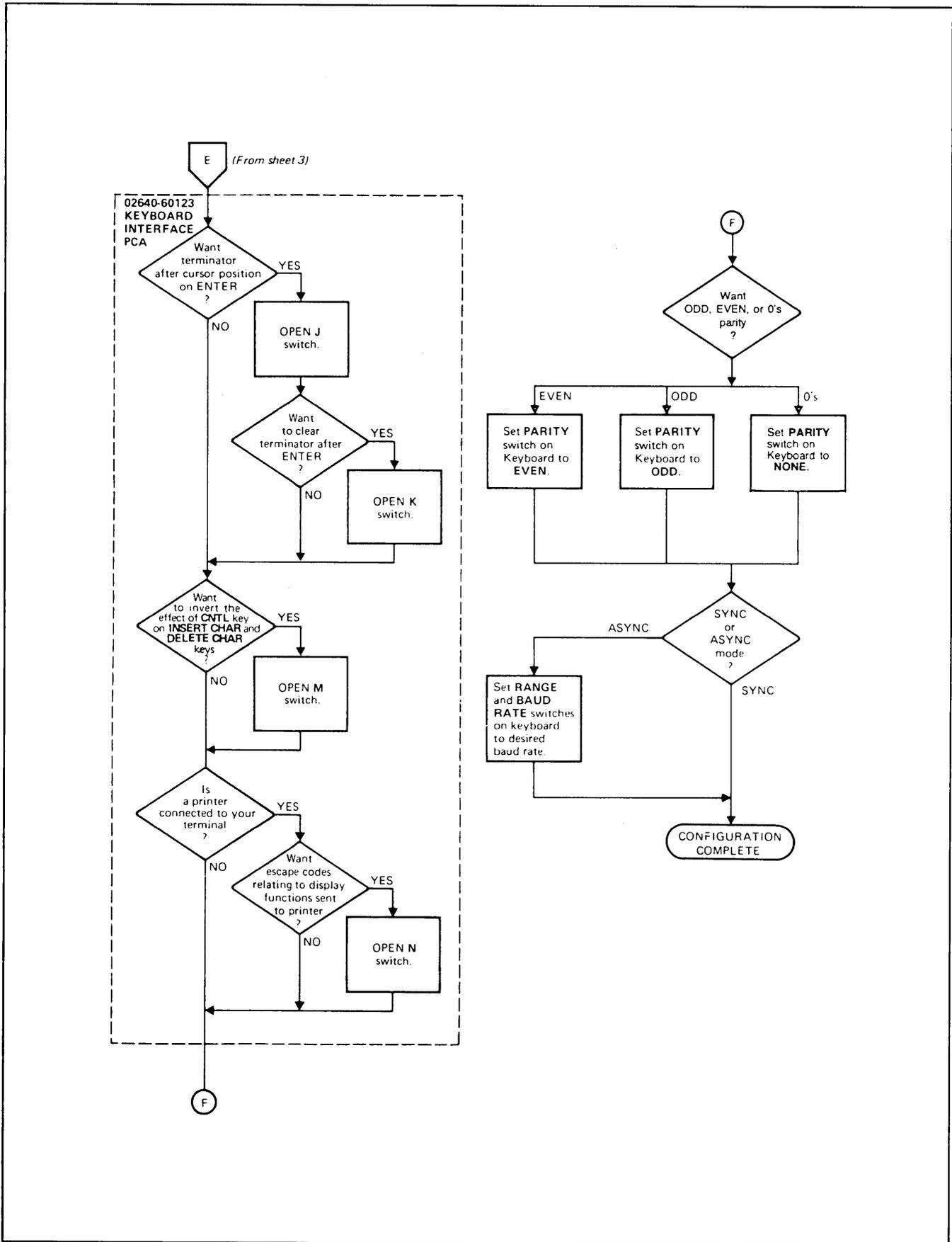
Figure 5-17. Multipoint Data Communications Configuration (Sheet 4 of 4)
