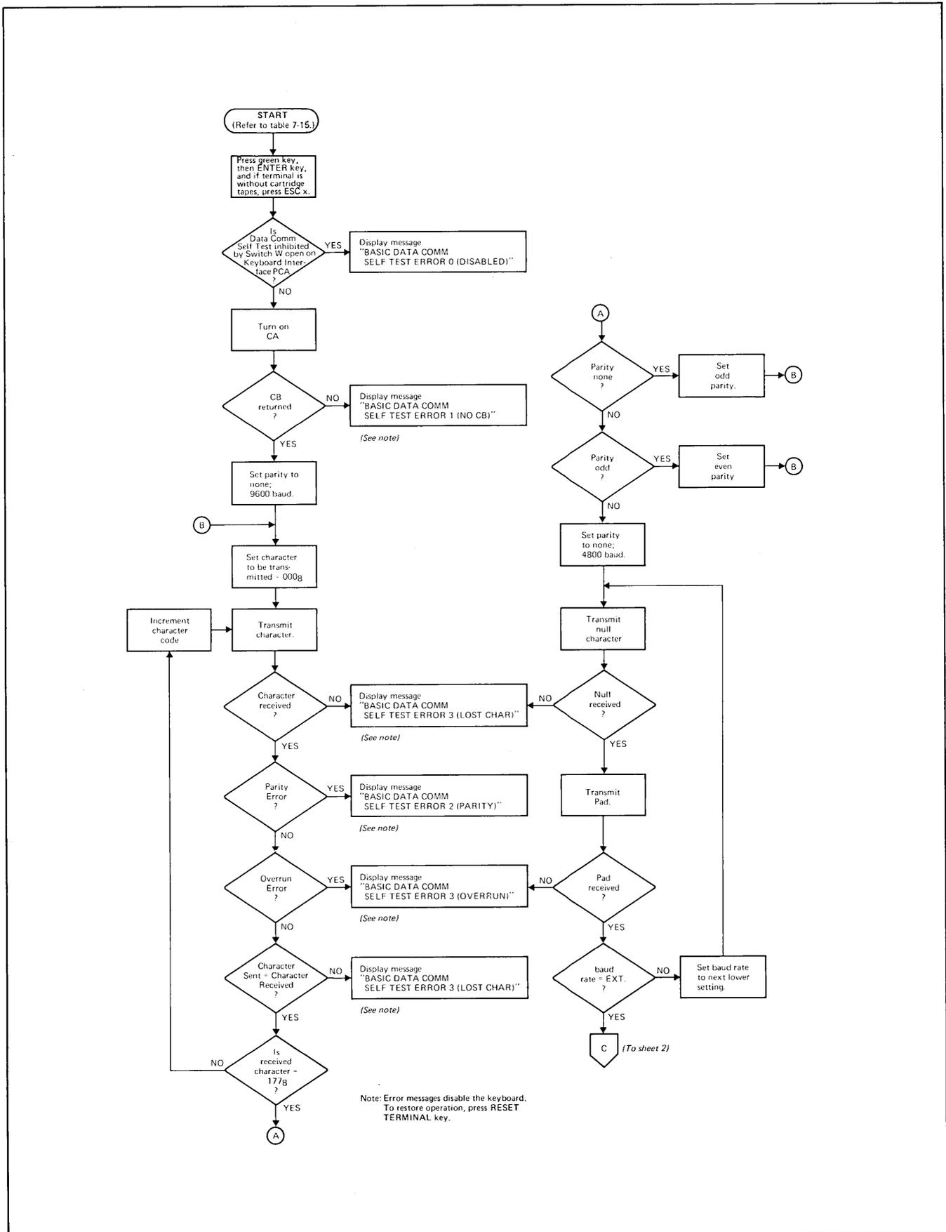
Figure 7-33. Basic Data Comm Self-Test Flowchart (Sheet 1 of 2)
