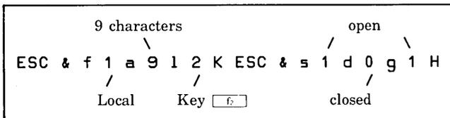
The soft keys can be used to hold log-on, program control, and log-off messages. This makes it easier for the terminal operator to use unfamiliar computer systems.
