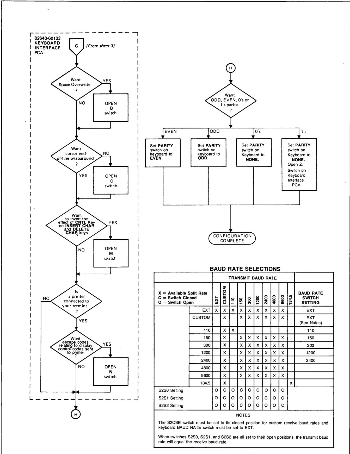
Figure 5-10. Point-to-Point Data Communications Configuration Flowchart (Sheet 4 of 4)
