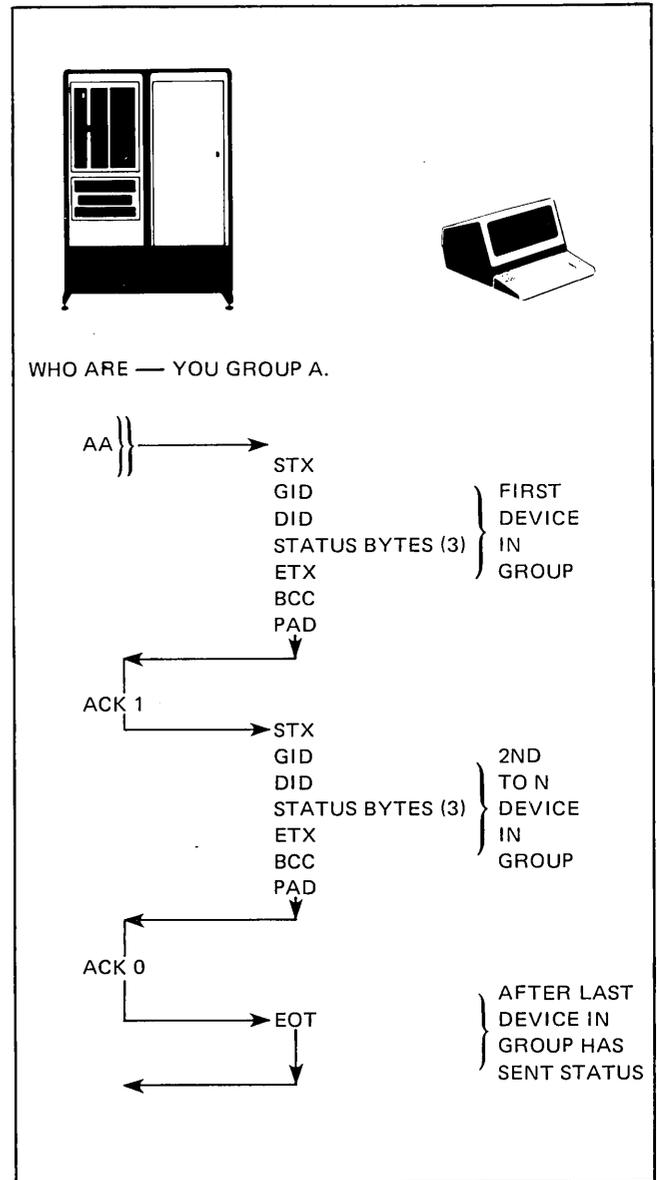
Figure 5-15. Typical Configuration Status Request and Response Sequence
