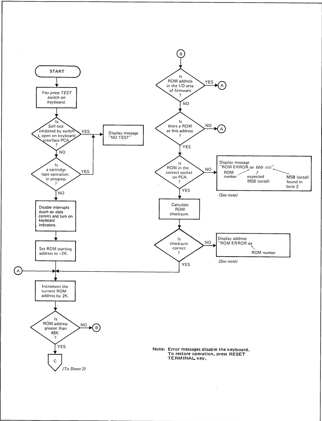
Figure 7-32. Basic Terminal Self-Test Flowchart (Sheet 1 of 3)
