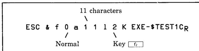
A third key could be used to log off of the system:
