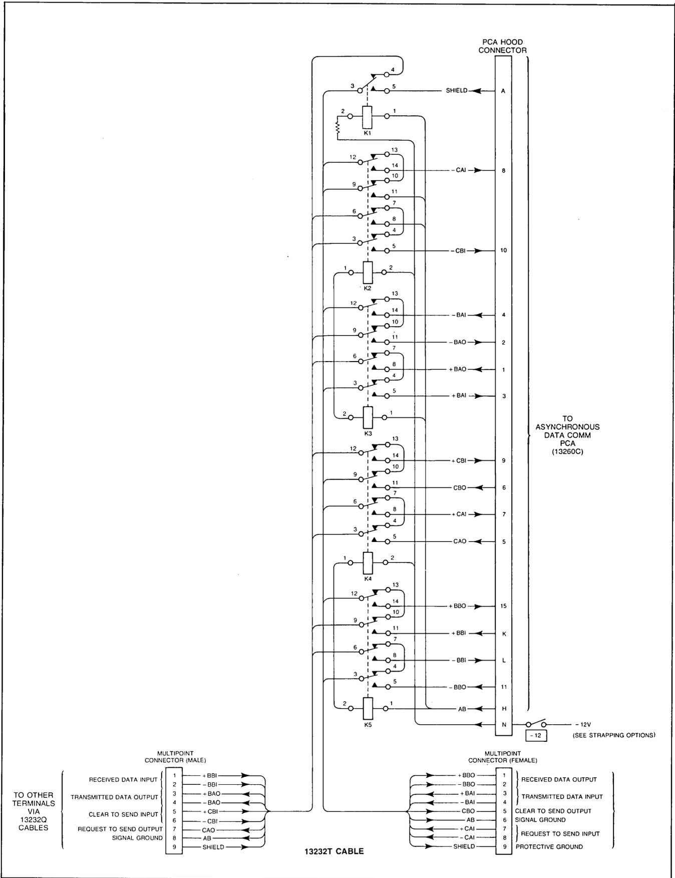
Figure 7-26. Power-Down-Protect Cabling for Asynchronous Multipoint Configuration
