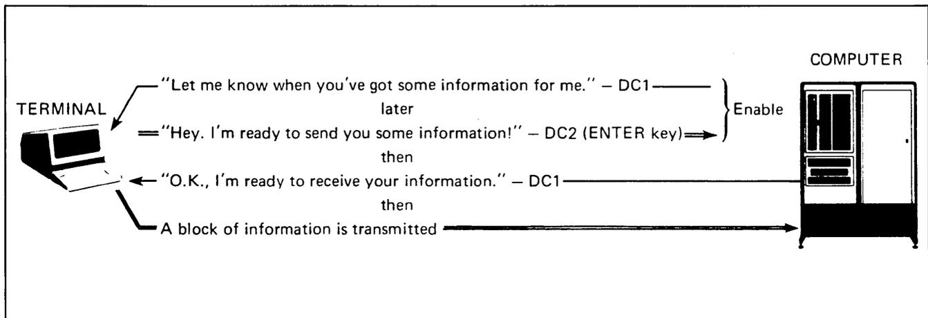
Figure 5-2. Block Transfer Enabled By The ENTER Key
