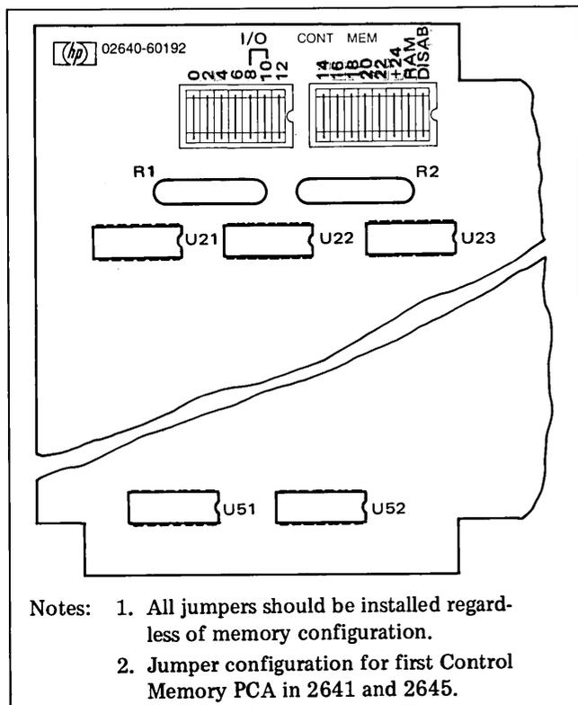
Figure 7-8. Control Memory PCA Jumper Socket Location
