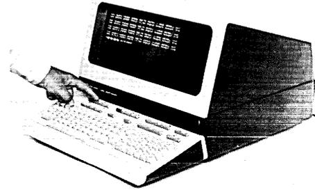
5. ( ) Firmly grasp mainframe top cover in one hand and release safety latch by pressing it inboard with your other hand. Then, using both hands, carefully lower top cover to its closed position.
