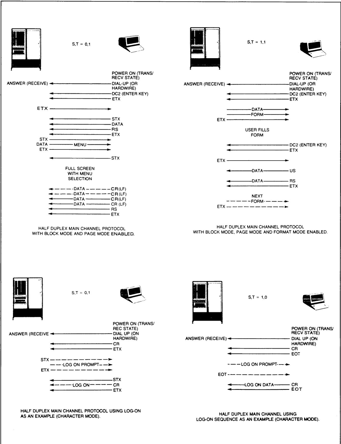
Figure 5-7. Simple Data Transfers Using Main Channel Protocol
