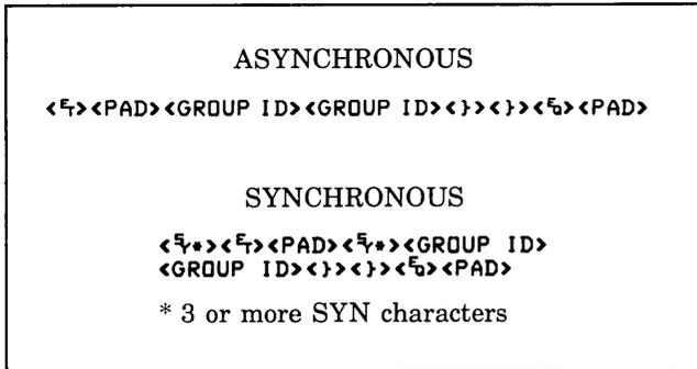
Three bytes of status information are returned for each responding terminal. Figure 5-15 shows a typical status request and responses from a terminal group.
