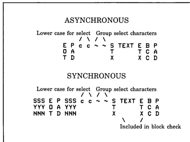
**Line Select.** A "line select" allows you to select all of the terminals on a communication line. This is also known as "Broadcast" mode. Both the group and device ID characters are replaced with tildes (~).
