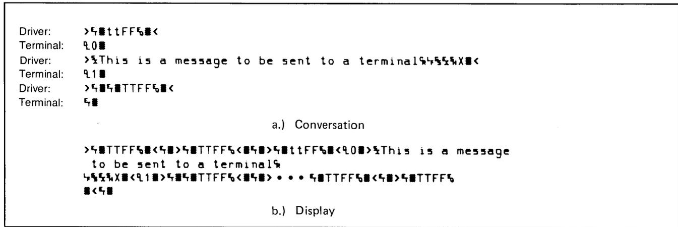
Figure 5-23. Sample Select Sequence Using Driver Mode
