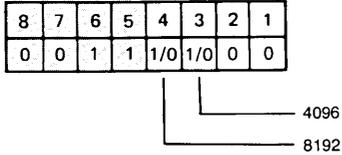
The amount of display memory (blocks of 1K) available in the terminal is returned. The amount can range from 4096 to 12,288 bytes.
