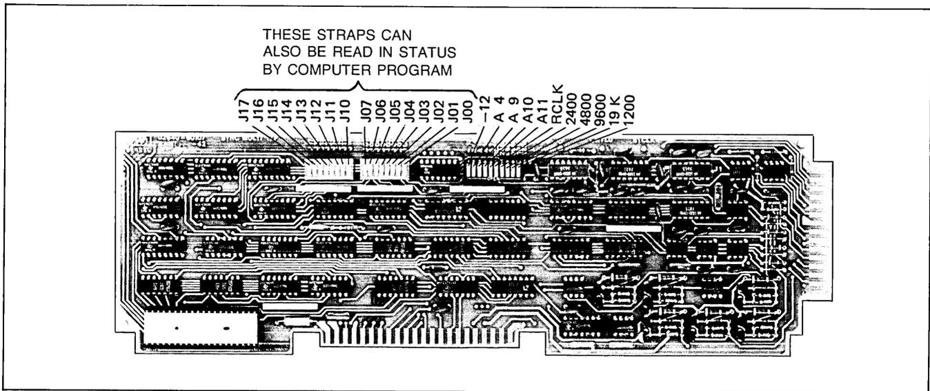
Figure 7-20. Synchronous Multipoint Communications PCA Strapping Options
