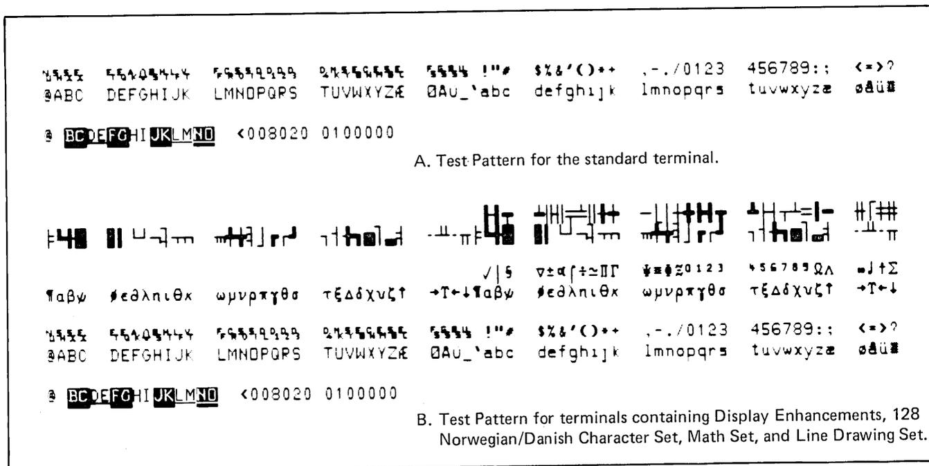
Figure 7-40. Basic Self-Test Patterns (HP 2645N)
