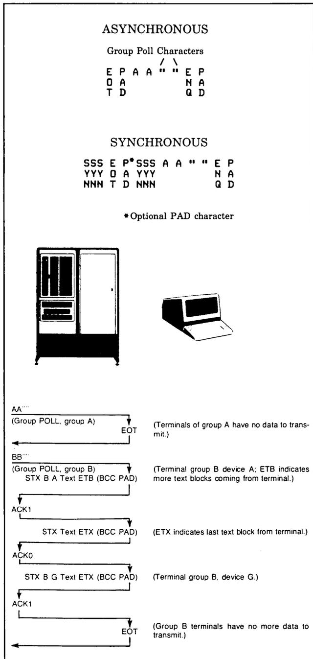
**Selection.** "Selection" occurs when the computer directs a specific terminal or group of terminals to accept a data transmission. The character sequences used in selection are the same as those used in polling. The only difference is that the lower case group ID characters are used. This is to tell the terminals that a selection is being sent instead of a poll. For example, to address the same device as in the polling example, the sequence would be as follows:
