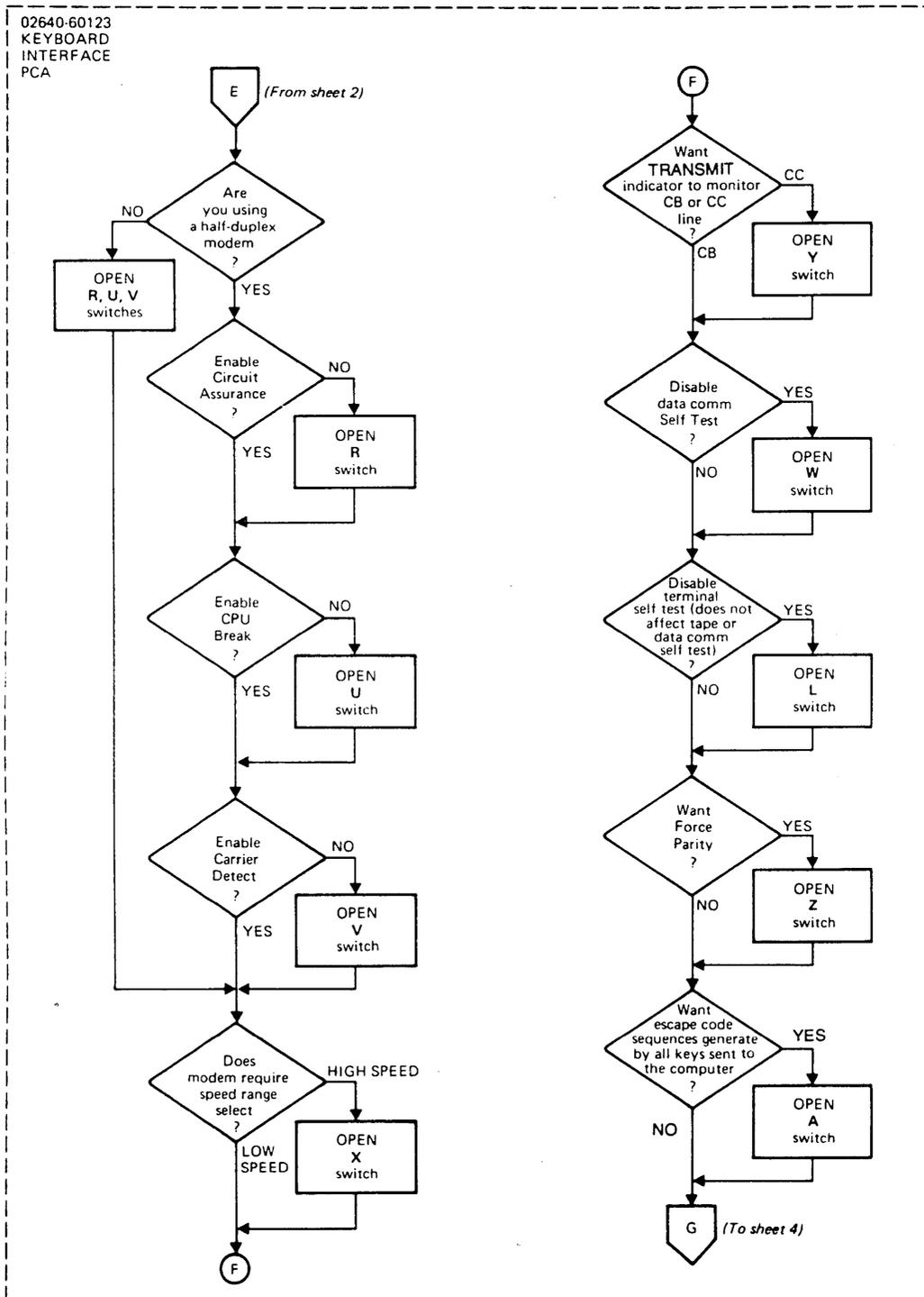
Figure 5-10. Point-to-Point Data Communications Configuration Flowchart (Sheet 3 of 4)
