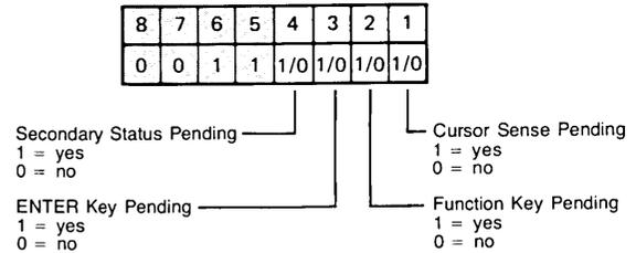
**BYTE 2 KEYBOARD INTERFACE SWITCHES (E-H)**
