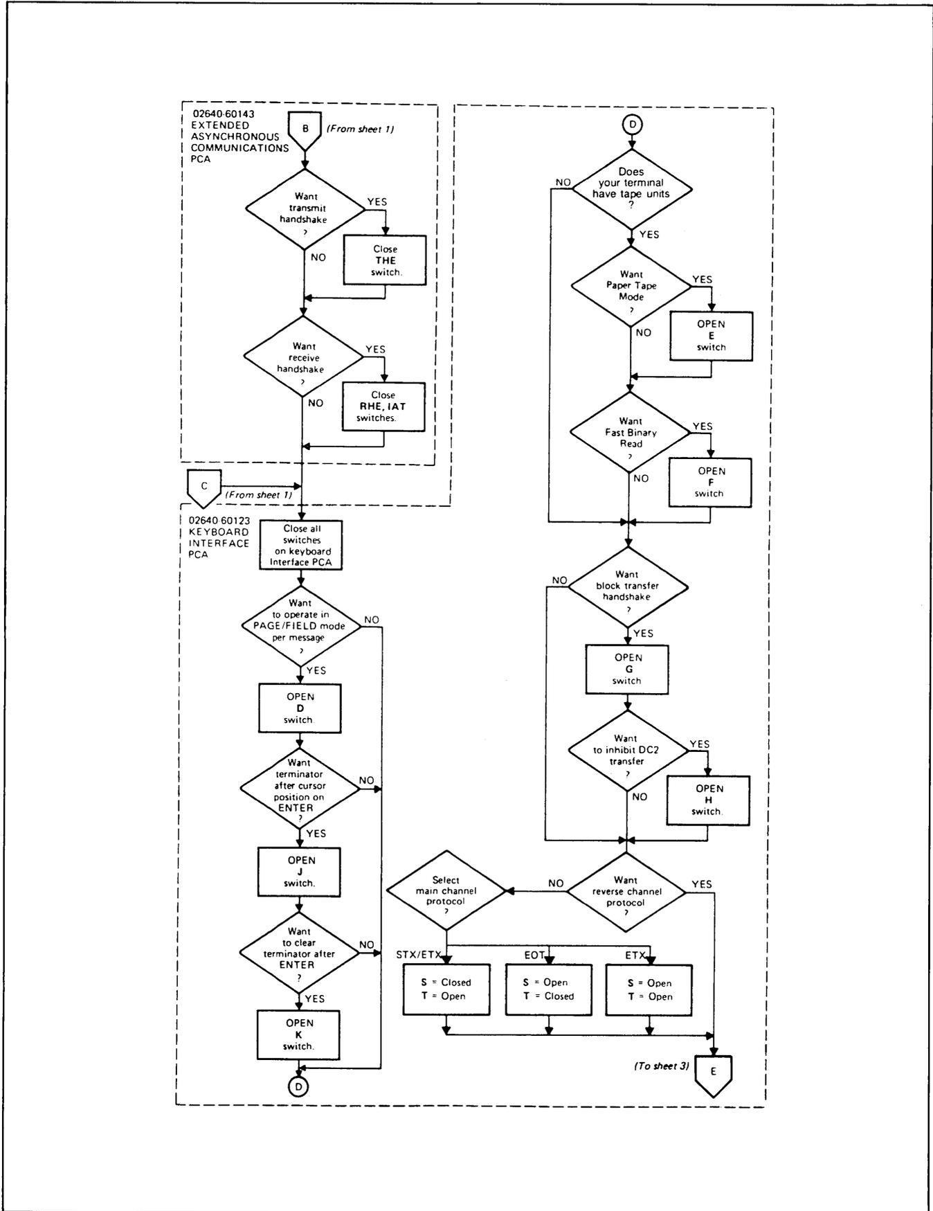
Figure 5-10. Point-to-Point Data Communications Configuration Flowchart (Sheet 2 of 4)
