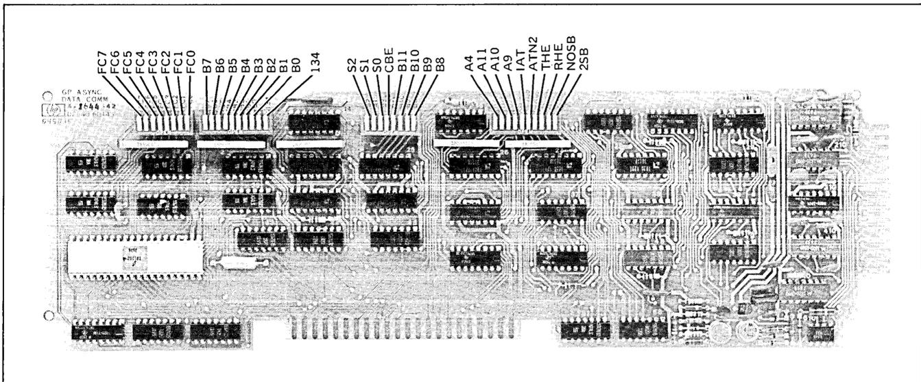
Figure 7-18. Extended Asynchronous Communications PCA Strapping Options
