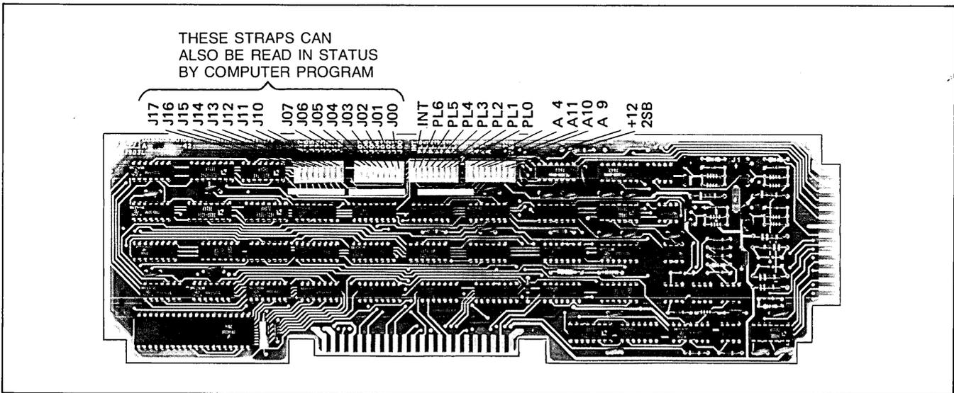
Figure 7-19. Asynchronous Multipoint Communications PCA Strapping Options
