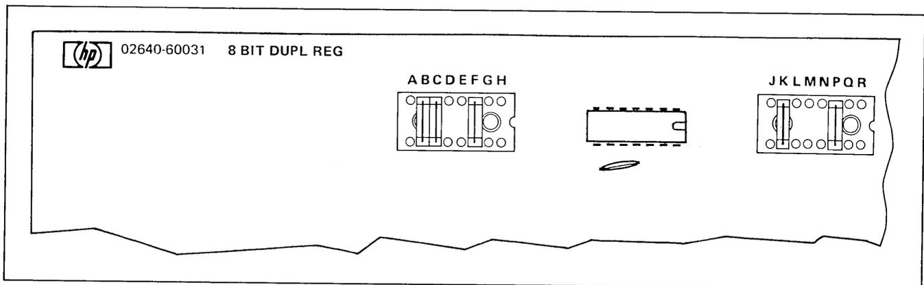
Figure 7-12. Terminal Duplex Register PCA Jumper Configuration
