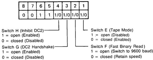
Refer to Section V for a detailed description of Keyboard Interface switches.
