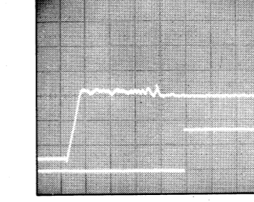
A12TP4 CURRENT COMMAND 5V/CM, 5 MSEC/CM
