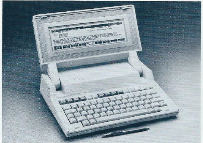
The Portable, a battery-powered personal computer from Hewlett-Packard, weighs nine pounds and measures 13 × 10 × 3 inches. It has built-in software packages and a screen with 16 lines by 80 characters.
