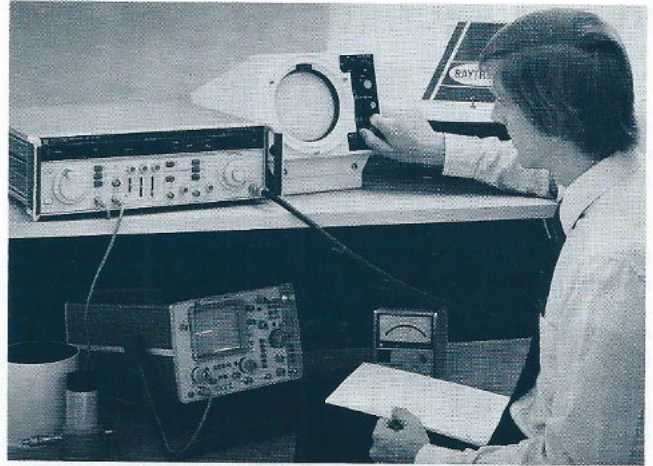
Option 001 for the HP 8683D Signal Generator provides 10 mW output power in the frequency-doubled band (6.5 to 13 GHz) as well as in the standard band.
