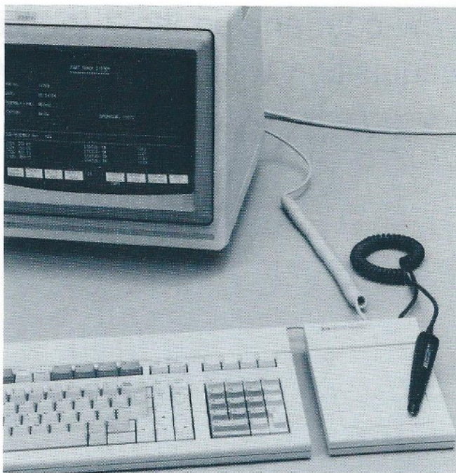
Offering a reliable alternative to keyboard data entry, the new HP 92915A Bar Code Reader adds bar code capabilities to the HP 150 Personal Computer and the HP 2392A Display Terminal.
