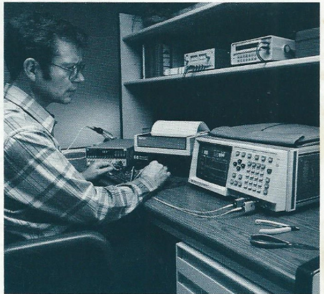
Competitively priced, the new HP 54200A/D Digitizing Oscilloscope can be used for capturing high-speed, single-shot and repetitive events at 200 megasamples per second.
