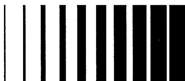
Figure 4-2 Examples of Line Widths
