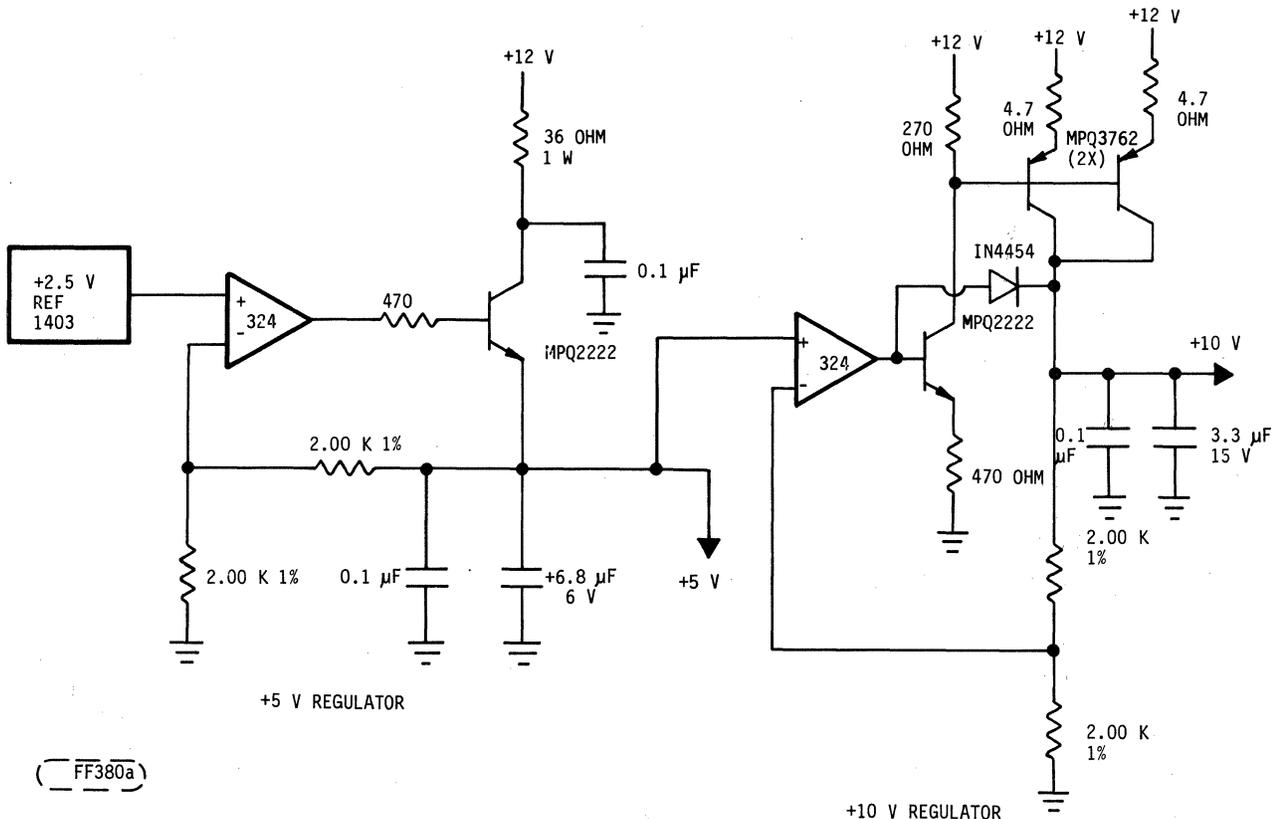
FIGURE 4-43. +5 AND +10 VOLT REGULATORS (CDC AND SEAGATE INTERFACES)
