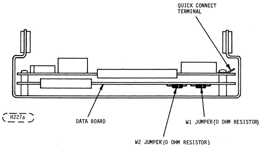
FIGURE 3-4C. PHYSICAL LOCATION OF W1 AND W2.
