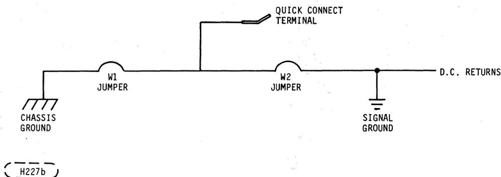
FIGURE 3-4D. SCHEMATIC DIAGRAM OF W1 AND W2.
