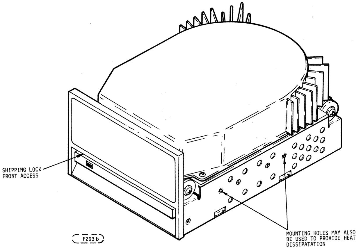
FIGURE 3-3. HEAT SINK MOUNTING HOLE LOCATION
