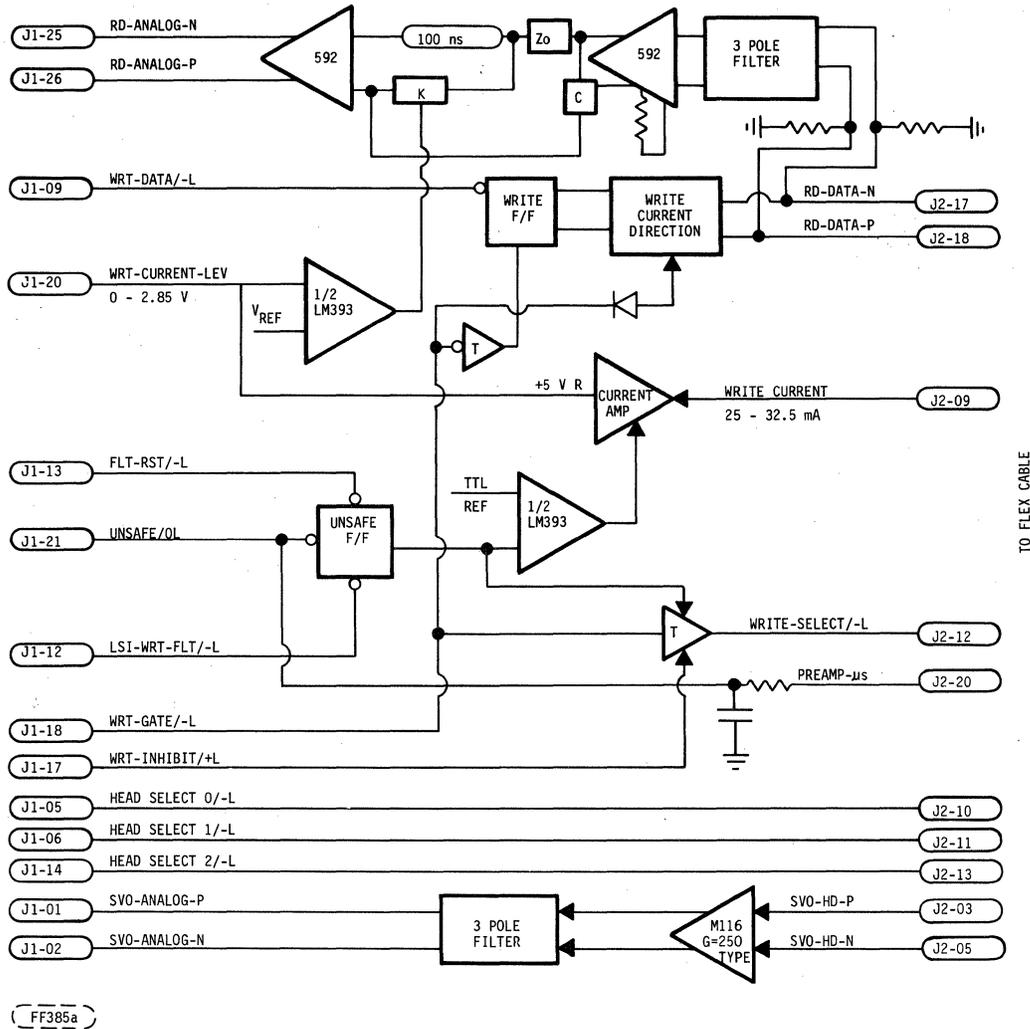
FIGURE 4-32. PRE-AMP BLOCK DIAGRAM (CDC INTERFACE)
