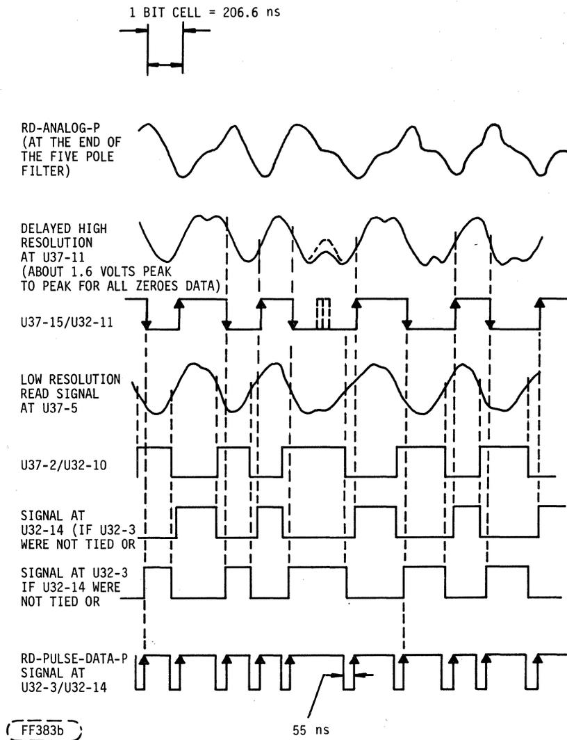
FIGURE 4-34. READ ANALOG TIMING DIAGRAM
