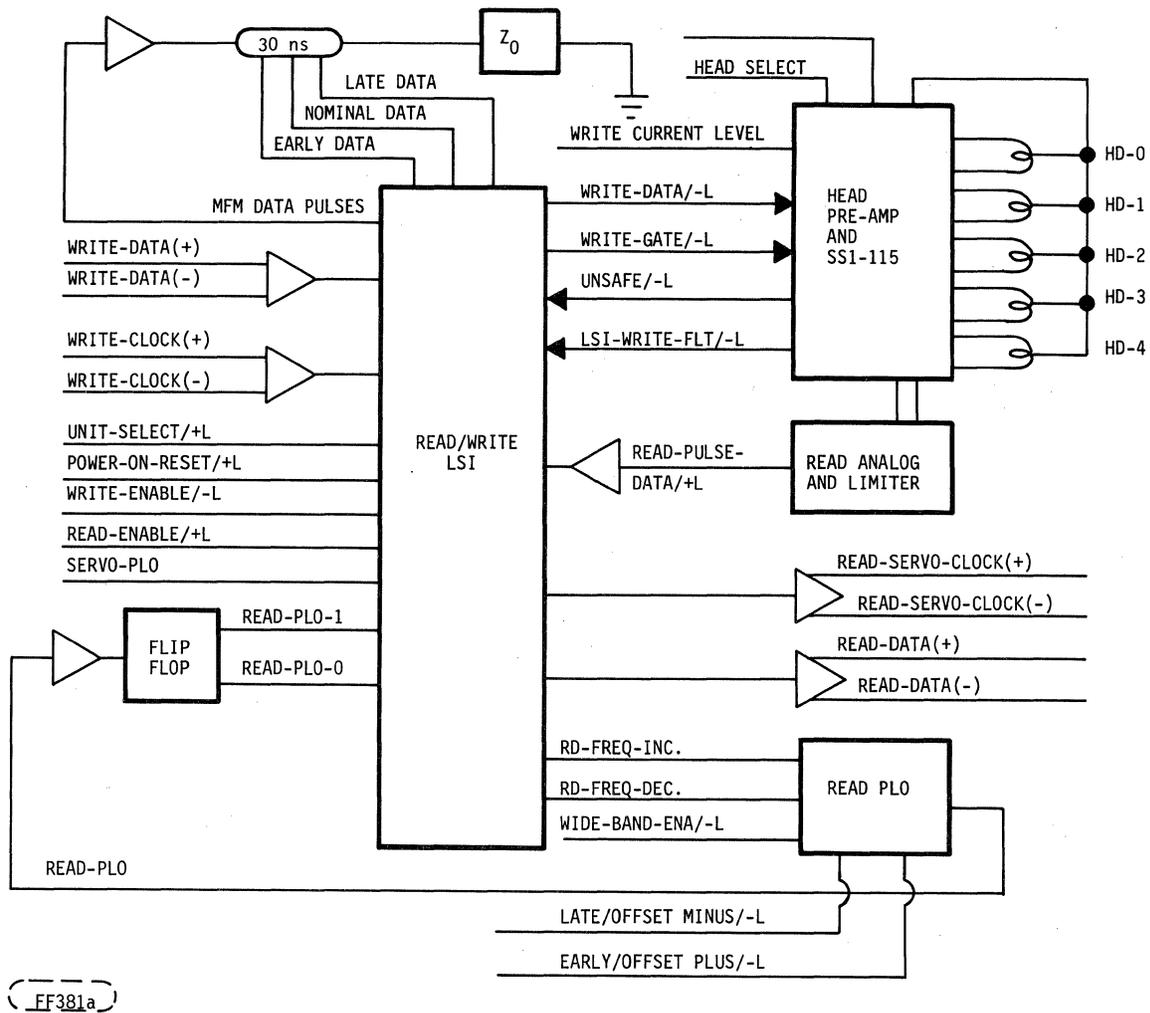
FIGURE 4-29. WREN I DATA BLOCK DIAGRAM (CDC INTERFACE)
