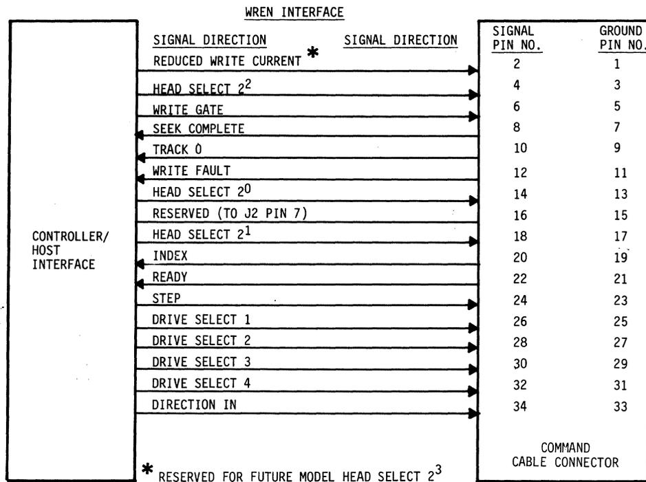
NOTE: ALL SIGNALS IN THE COMMAND CABLE ARE SINGLE ENDED SIGNALS.
