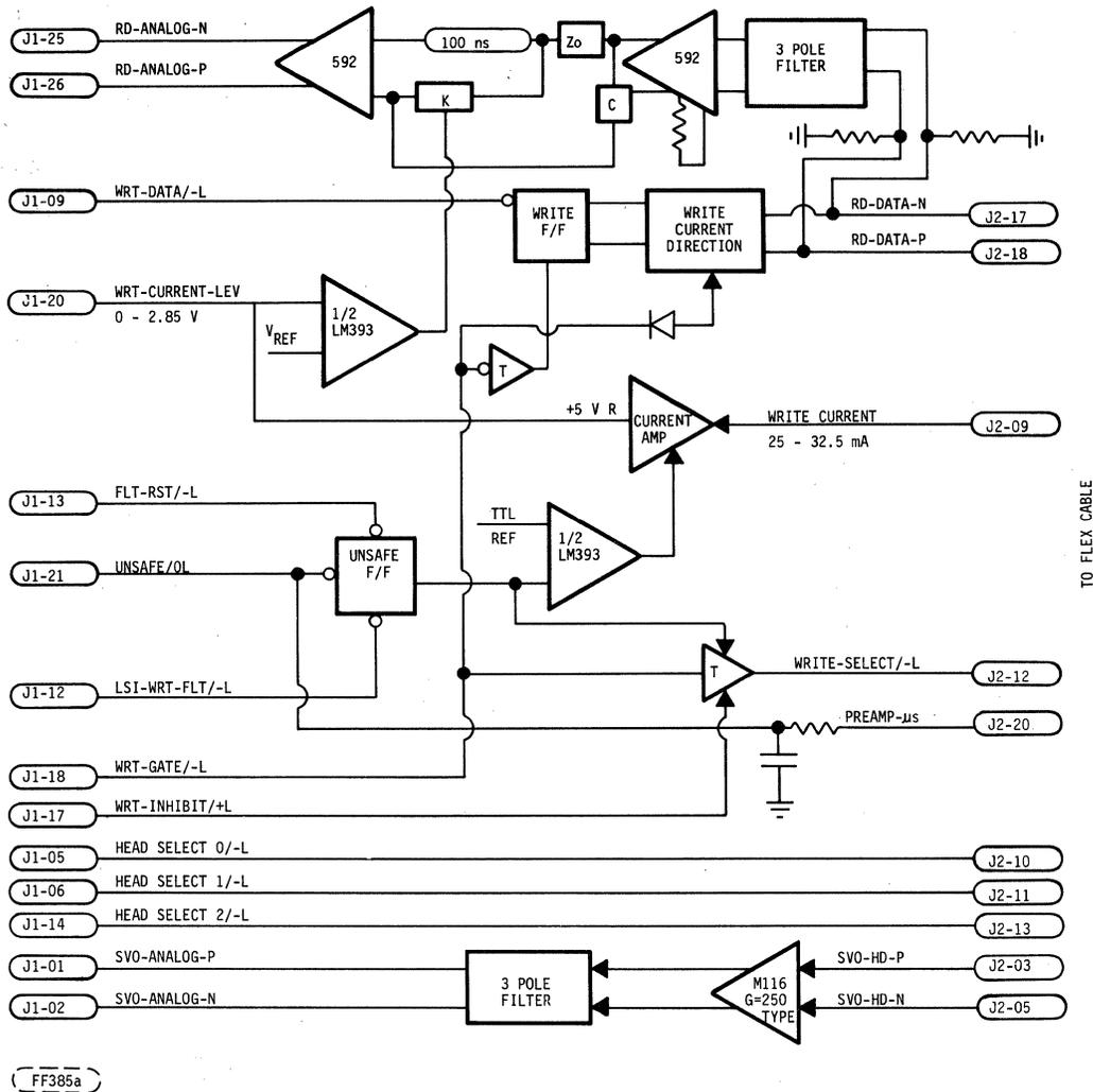
FIGURE 4-35. PRE-AMP BLOCK DIAGRAM (CDC INTERFACE)
