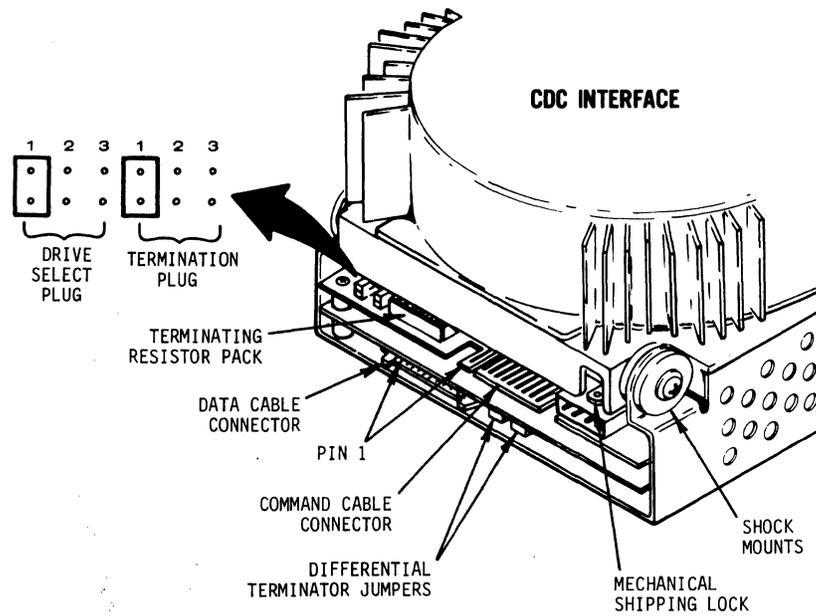
FIGURE 3-4A. COMMAND, DATA, AND POWER CABLE REQUIREMENTS FOR MODEL 9415-3
