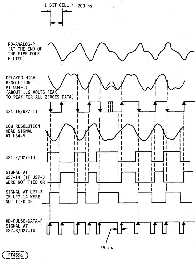
FIGURE 4-37. READ ANALOG TIMING DIAGRAM (SEAGATE INTERFACE)
