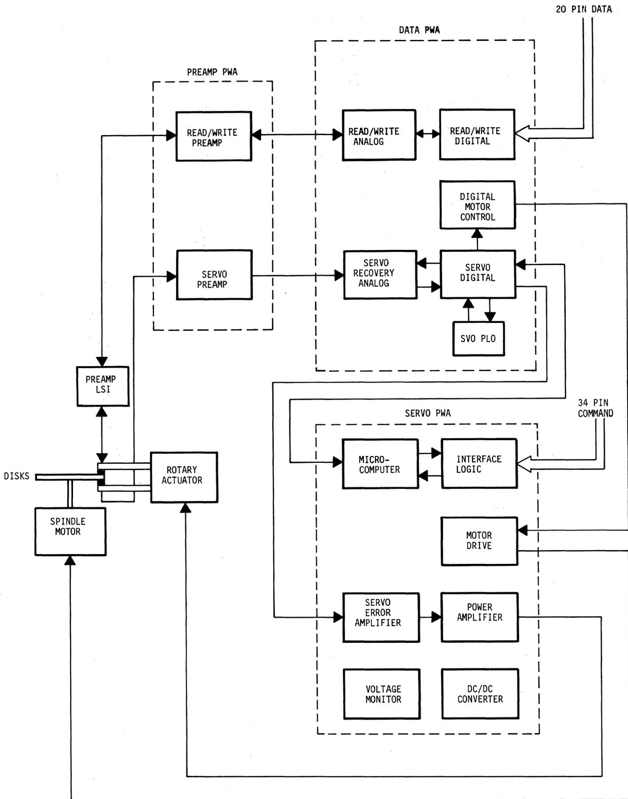
FIGURE 5-1. WREN I BLOCK DIAGRAM
