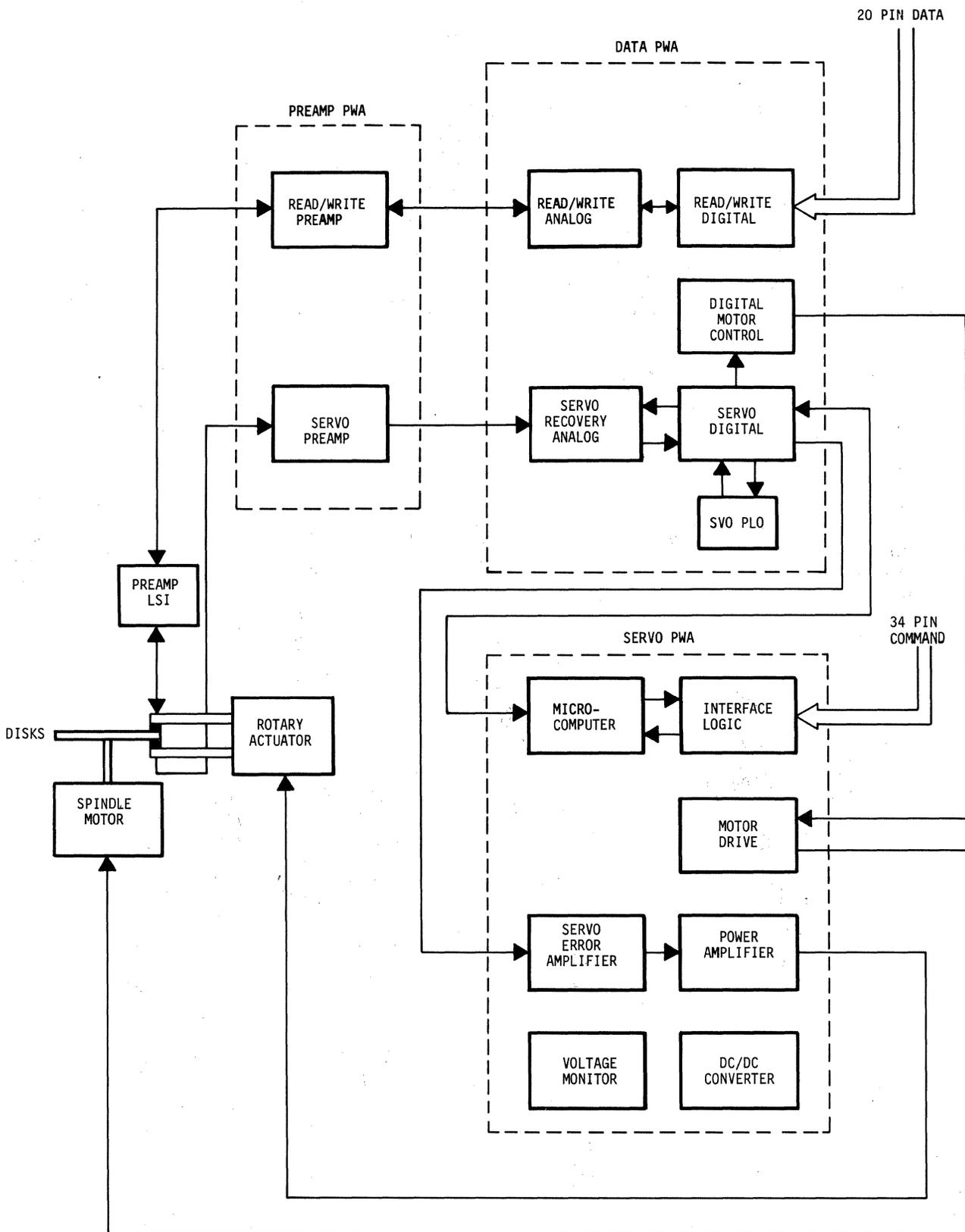
(FF378a) FIGURE 4-1. WREN I GENERAL BLOCK DIAGRAM (CDC AND SEAGATE INTERFACES)
