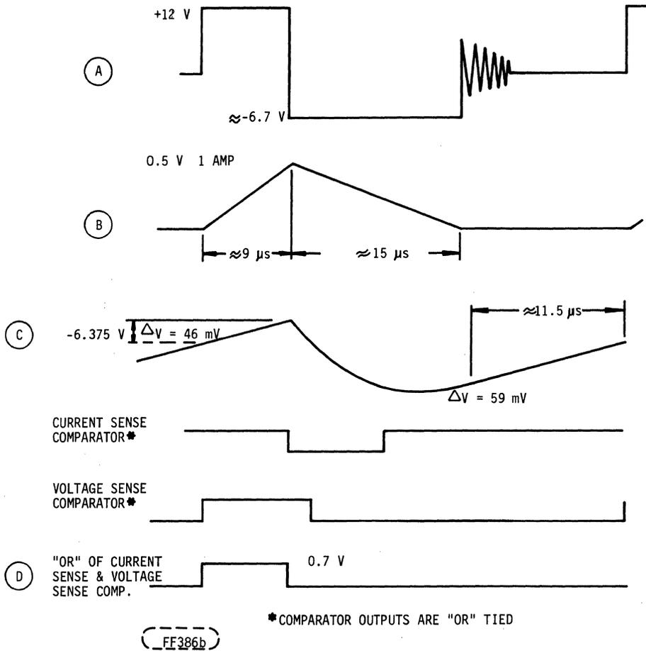
FIGURE 4-42. DC-DC CONVERTER WAVEFORMS (CDC AND SEAGATE INTERFACES)
