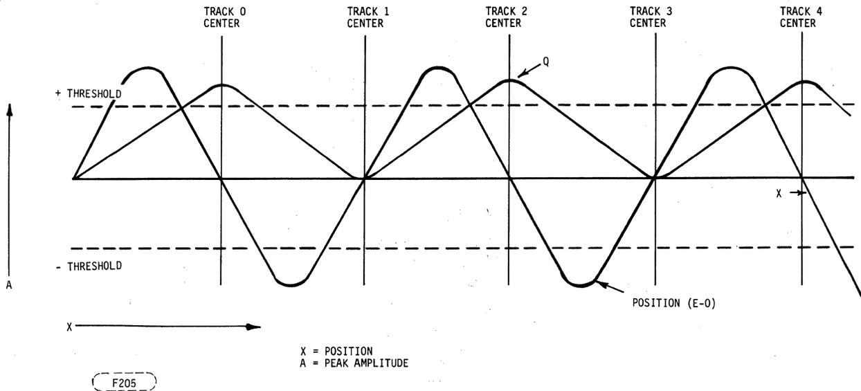
**FIGURE 4-26. DERIVED POSITION AND QUADRATURE SIGNALS
