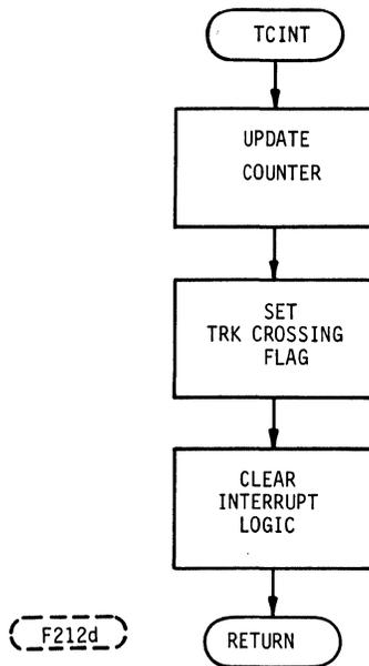
FIGURE 4-19. TRACK CROSSING INTERRUPT (CDC AND SEAGATE INTERFACES)
