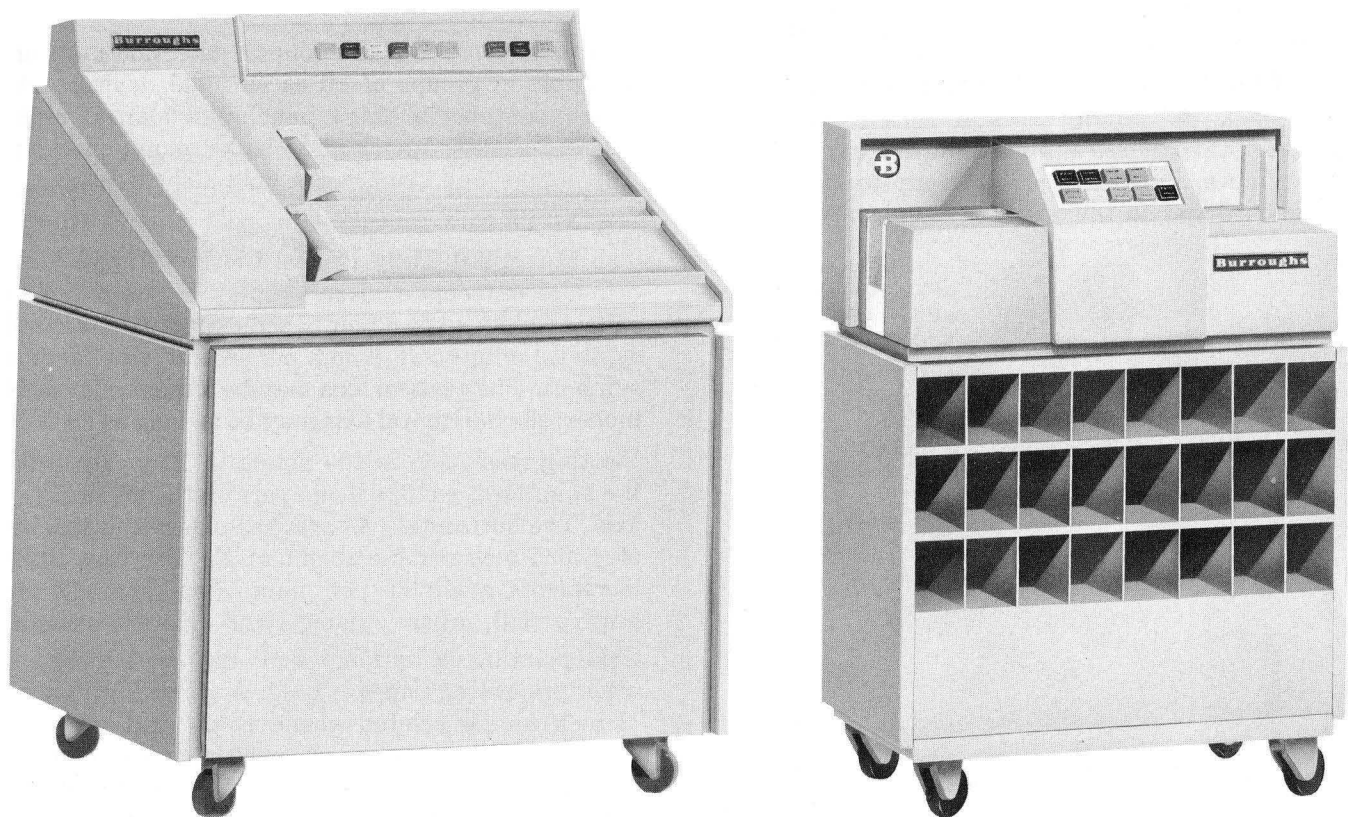
Figure 5-10. 800 CPM Reader and Program Card Reader
