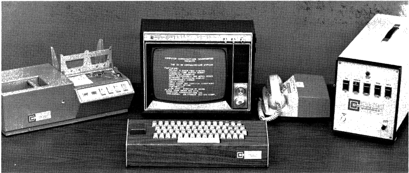
Figure 1. CC-30 Communications Station including CC-300 Model II Television Receiver, CC-303 Model III Alphanumeric Keyboard, and CC-301 Model II TV Display Controller.
