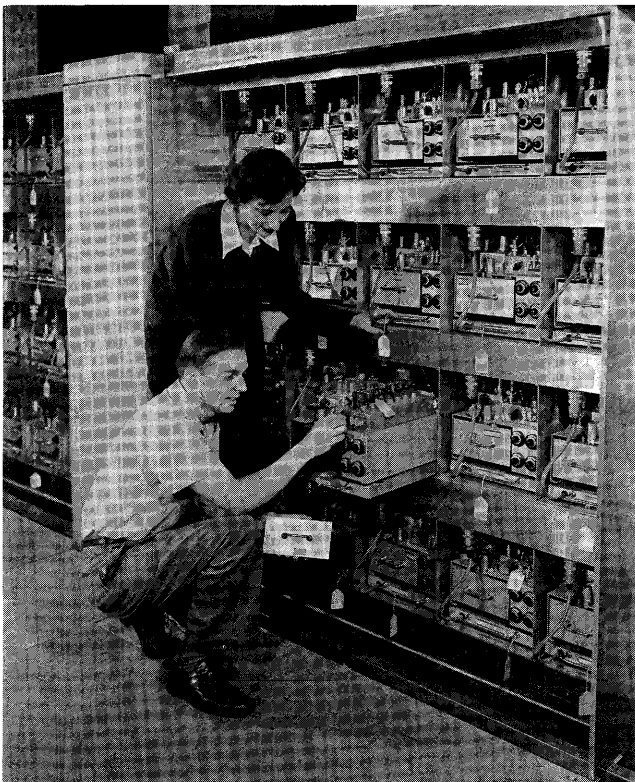
Figure 5—Margaret Butler and Bud Klein servicing a troublesome memory unit
