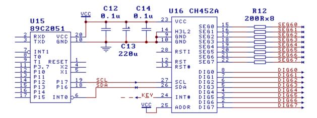
8.3. Drive Common Cathode LED Nixie tube (as shown below)
