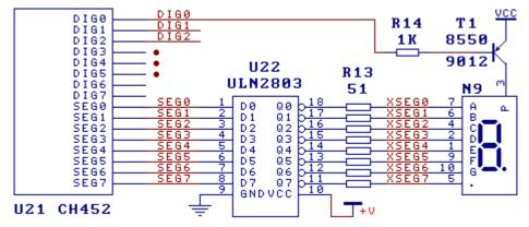
The figure below is a simple large current common anode drive application circuit. Set the word drive DIG output polarity of CH452 as "active at high level", and use N-MOSFET to realize voltage drop and large current drive simultaneously. Usually the current limiting resistor R13 for segment drive can be removed.
