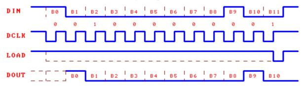
The figure above is a waveform diagram of the 12-bit data sent by the MCU to CH452 through a 4-line serial interface when the keyboard scan function is not enabled. The data is 00100000001B, and the low level pulse of LOAD can be wider, which is represented by the dotted line in the figure.
