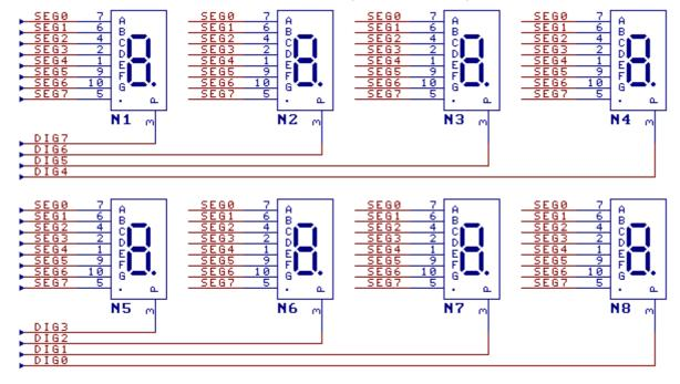
CH452 can drive 8 common cathode LED Nixie tubes dynamically. After the pins on the same segments of all LED Nixie tubes are connected in parallel (segments A-G and decimal point), they are connected with the segment drive pins SEG0-SEG7 of CH452 through a series current limiting resistors R1 (or R12). The cathodes of each LED Nixie tube are driven by the pins DIG0~DIG7 of CH452 respectively.
